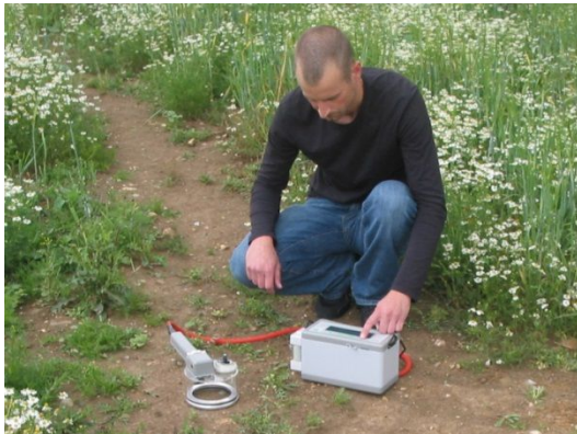
Measuring soil respiration in the field, February 2014 by Steveadcuk, Creative Commons
