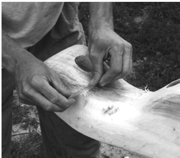
Figure 16: A shard of broken glass brings the surface to a hard smooth finish.
