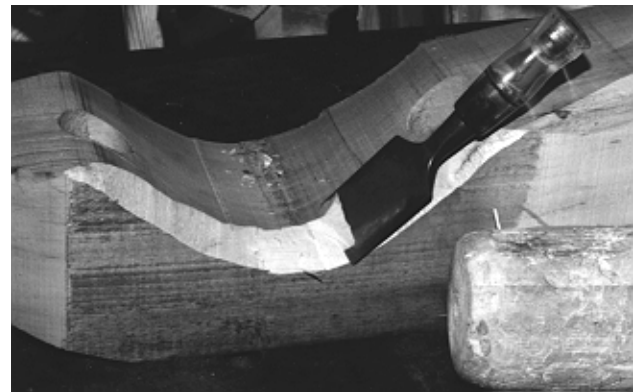
Figure 14: A large chisel and mallet being used to shape the neck seat of a yoke beam.
