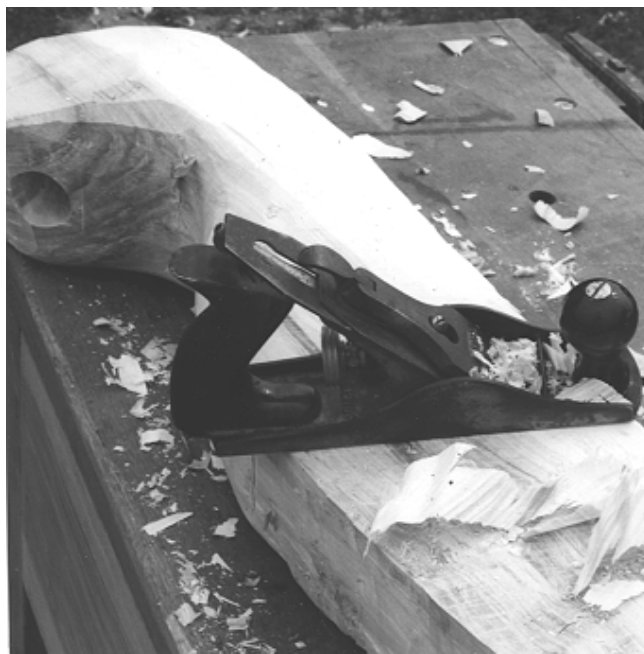
Figure 17: A hand plane is a good choice for quickly smoothing the sides of the beam. It removes stock quickly when pushed across the grain.
