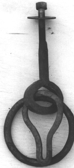
Figure 36: For small yokes a staple with a single threaded stem and a closed bulb works well.
