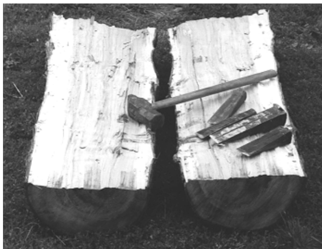
Figure 5: A yoke beam split from a large log is less likely to check when drying than one made from a smaller full log.
