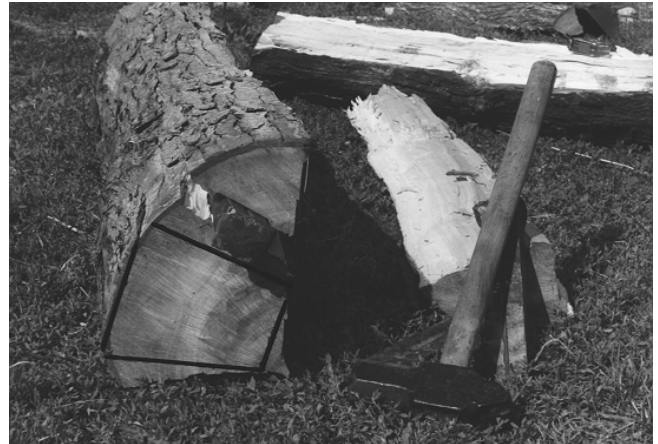
Figure 8: Mark the cross section of the beam on the end of the log and then split outside your lines.
