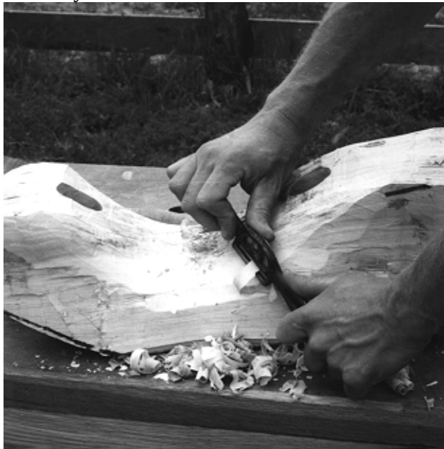
Figure 15: A spoke shave efficiently smooths the neck seat of a yoke beam.
