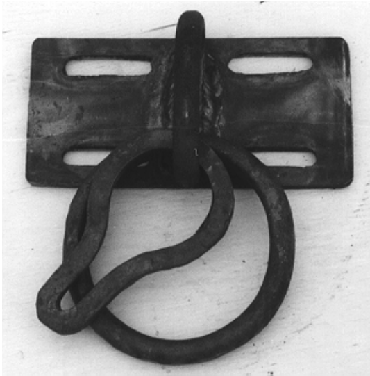
Figure 35: The bottom plate of an adjustable staple can be fabricated in most metal shops.
