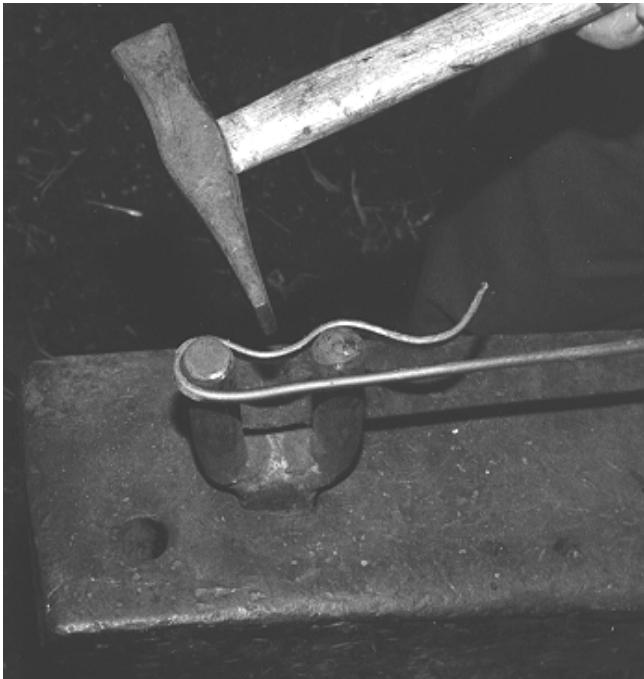
Figure 25: Bow pins are shaped on a bending fork set in the hardy hole of the anvil.
