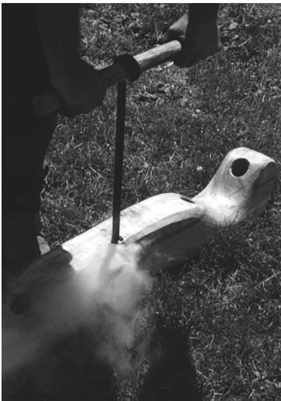
Figure 32: Holes for the staple are squared with a heated square bar of steel.
