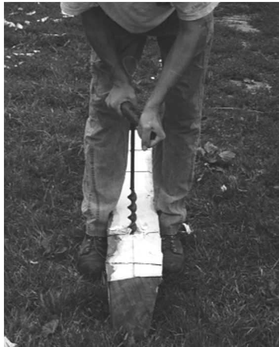
Figure 11: A “T”-handled auger bores the bow holes in the yoke beam.
