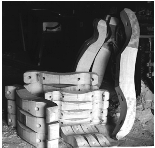
Figure 13: Yoke blanks cut out with a band saw in Tillers' production shop.
